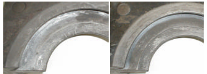
Figure 13: The mould lifetime prolongation by the mould cracks elimination.
