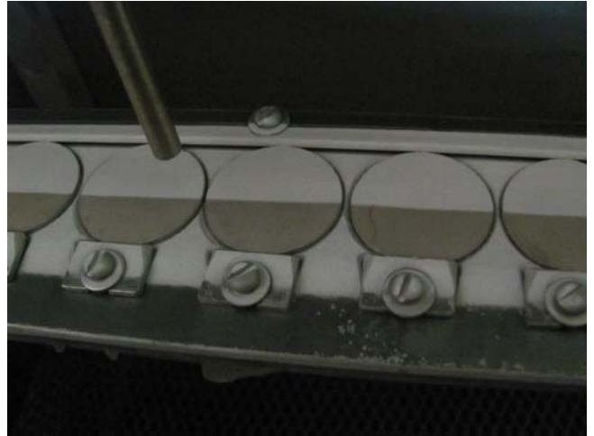
Fig. 6. Spraying of aluminum barrier layer to the surface of Bi 2 SbTe semiconductor plates.
