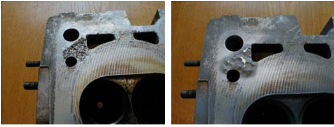
Figure 9: Restoration of corrosion defect on car engine by spraying aluminum based powder mixture.
