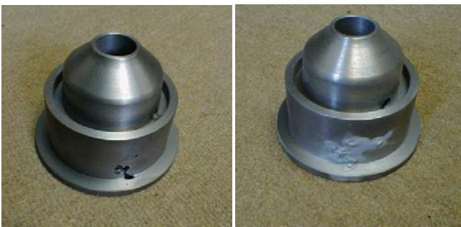
Figure 10: Filling the casting defect on the steel part by aluminum based coating.
