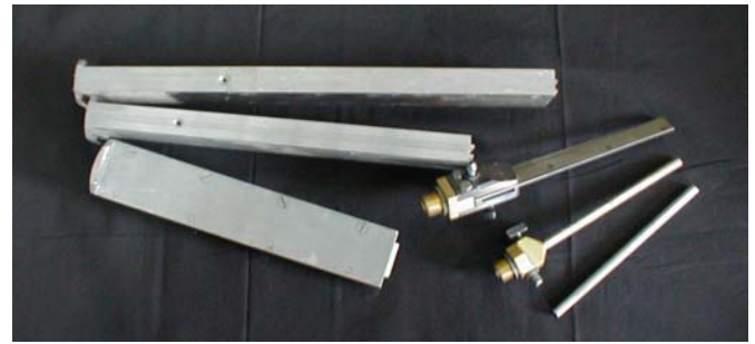
Figure 7: Former and modern DYMET nozzles.
