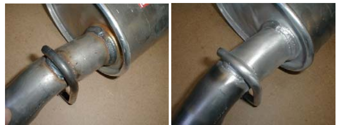
Figure 12: Corrosion protection coating at welding lines.
