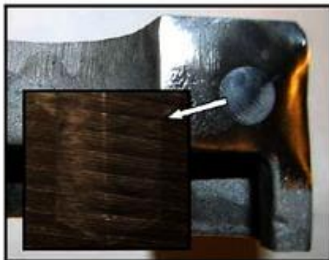
Fig. 4. Repaired casting defect by using LPCS Zn+Al+Al 2 O 3 coating. Digital camera image.
