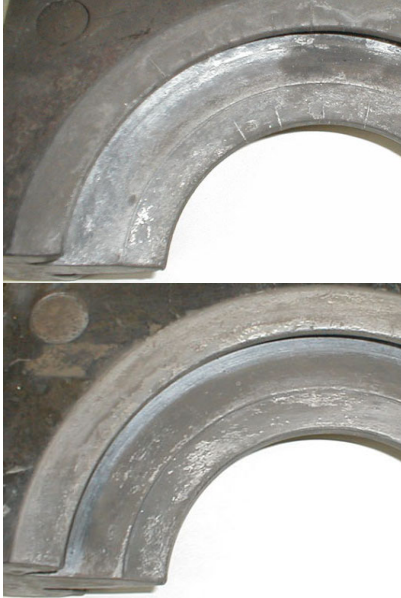
Figure 13: The mould lifetime prolongation by the mould cracks elimination.
