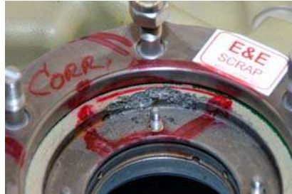
Fig. 3. Corrosion damage in magnesium alloy castings used in rotorcraft.
