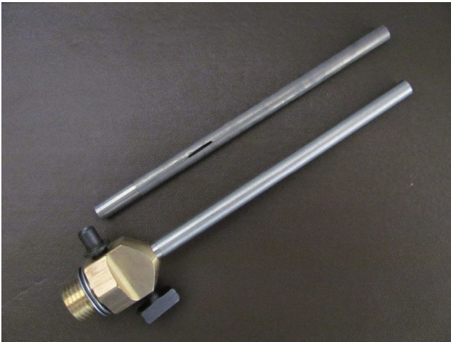
Figure 8: Nozzle with the steel insert and the eroded insert.
