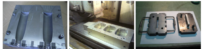
Figure 2: Elimination of defects at casting moulds.
