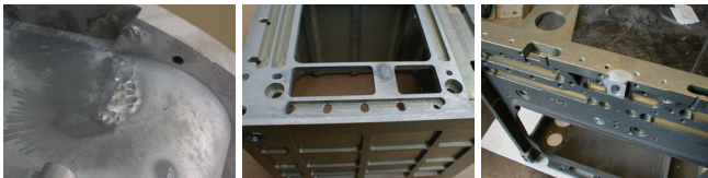
Figure 4: Casting and machining defects correction.
