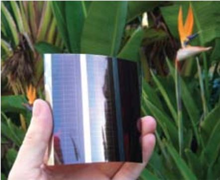
Figure 4: Printed organic solar cell where each of the layers has been printed, including the metal electrodes.
