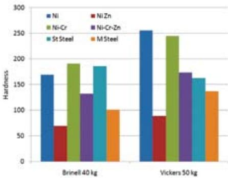
Figure 2 Brinell and Vickers hardness of the Dymet coatings in comparison with stainless and mild steels
