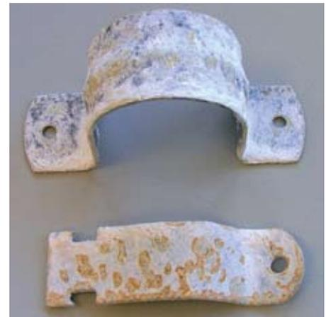
Figure 3B The samples 6 and 7 after the salt spray test
