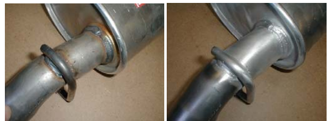
Figure 12: Corrosion protection coating at welding lines.
