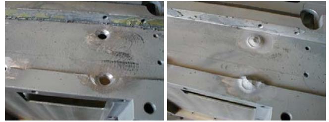
Figure 11: The sealing of the holes in the aluminum case.
