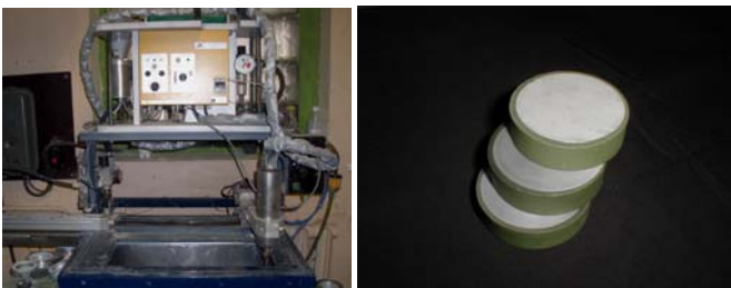
Figure 14: Simple automatic system for ceramic surface metallization and ready to use varistors.
