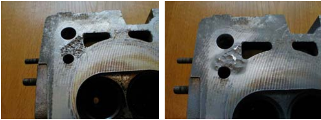
Figure 9: Restoration of corrosion defect on car engine by spraying aluminum based powder mixture.
