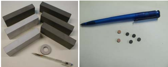
Fig. 8. Magnet sensors and UHF ferrites coated by low pressure cold spray process.
