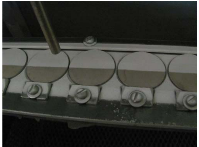
Fig. 6. Spraying of aluminum barrier layer to the surface of \text{Bi}_2\text{SbTe} semiconductor plates.
